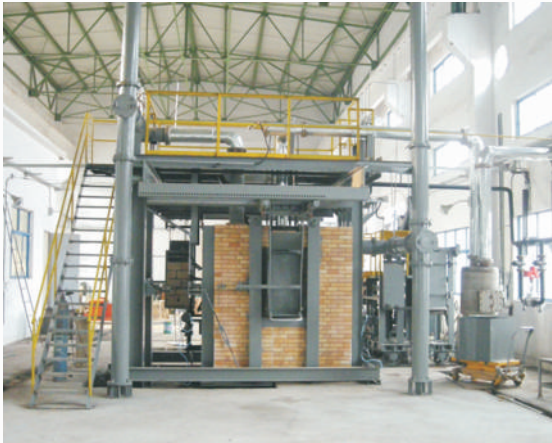
200kg煤气加热试验焦炉 200kg Gas heating test coke oven
