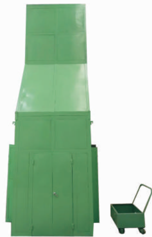
全自动落下装置 Automatic coke dropping strength measuring device
