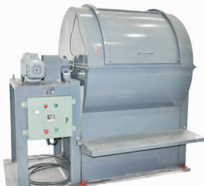
MK-8环保型焦炭机械强度测定转鼓 MK-8 Coke mechanical strength measurement drum (environment protection type)
