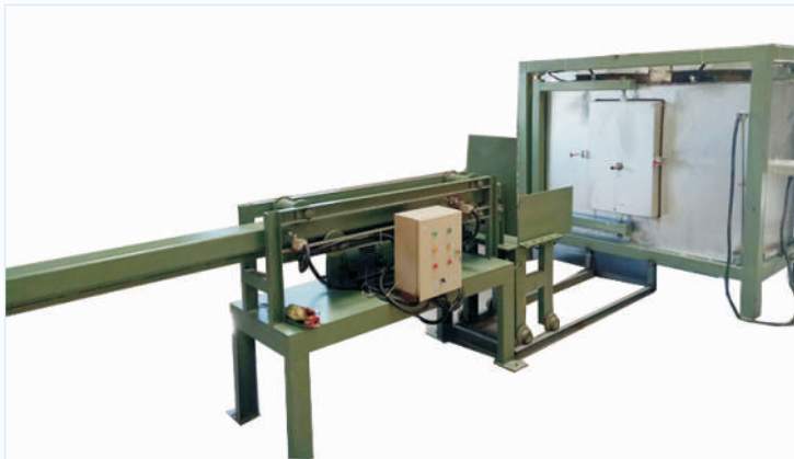
侧装焦炉 Side coke oven
