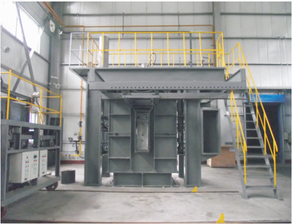
400kg电加热试验焦炉 400kg Electrical heating test coke oven
